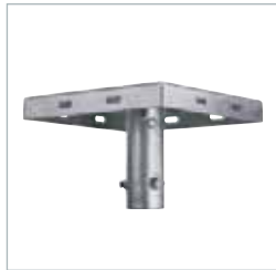
60240 AKRON 4 Hot deep galvanized sheet steel accessory for max 4 floodlights 400W max fixing on 60 mm diam. pole.
