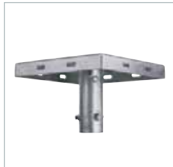
60240 AKRON 4 Hot deep galvanized sheet steel accessory for max 4 floodlights 400W max fixing on 60 mm diam. pole.
